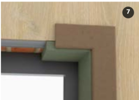
Door finish with MDF and door frame
