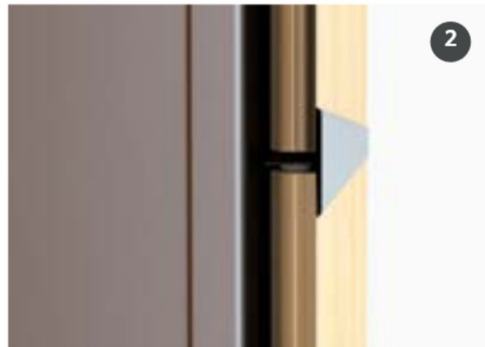
Finishing with aluminium T-profile
