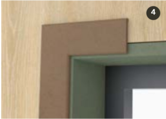
Window finish with MDF and window frame
