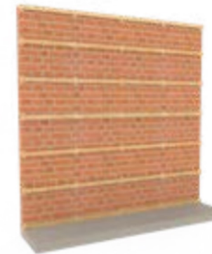
Timber battens straight onto wall
